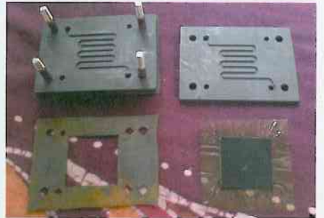
Above: A computer-generated impression of what the Version 2 UAV will look like. Below: A homemade four-cell stack showing the bipolar plates that route the hydrogen (through the snake-like gas flow fields) over the membrane electrode assembly.
